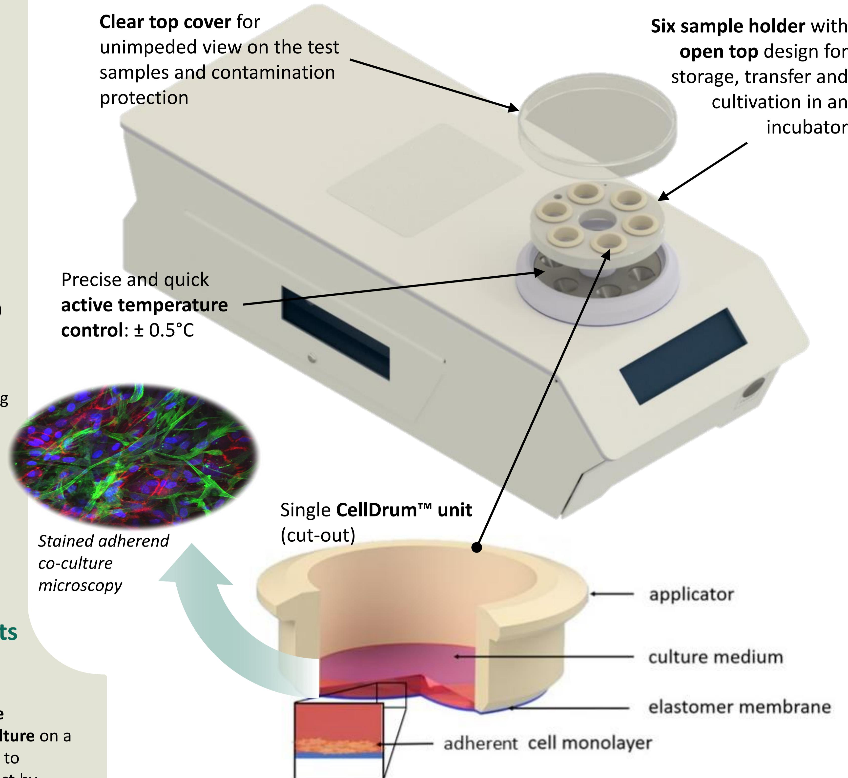
CFA<sub>ref</sub> allows consecutive tensile stress measurements of up to 6 CellDrum™ units. The cell cultures within can have contractions with “high” or “low” velocity. For both cases different program functions are used. The adherent cells are **cultured on exceptionally thin PDMS membranes** (3.4-4 µm) as cell culture substrate over several days, allowing cell culture **approaches closer to in-vivo environments**.
